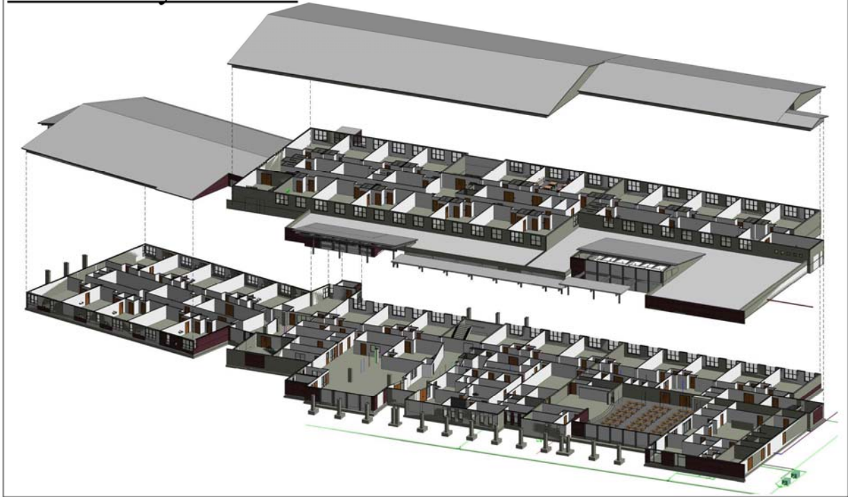
Figure C-1. 3D sections of Elementary School
